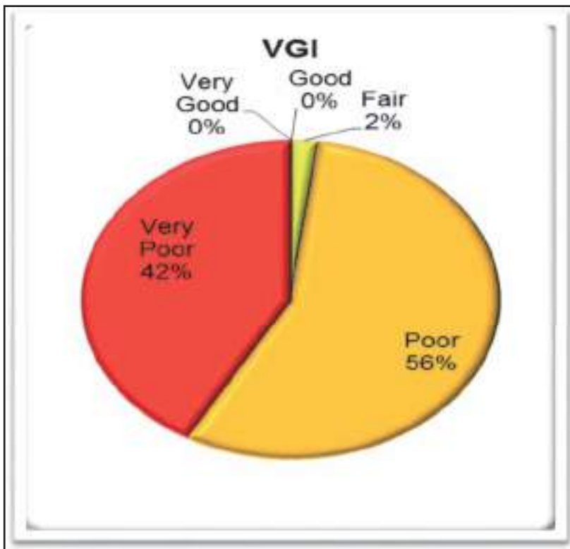
Figure 3: Network-level distribution of unsurfaced road conditions
