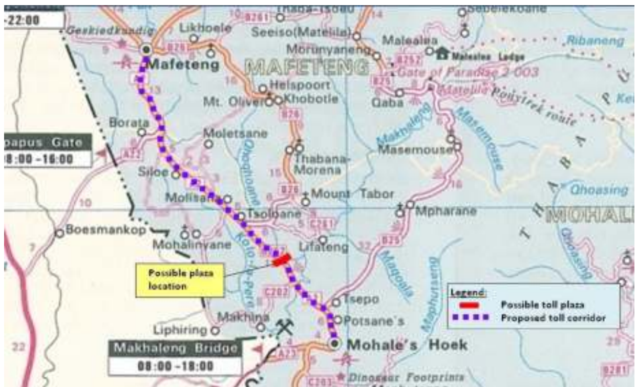
Figure EXEC 4-6: Proposed Toll Section 6: Route A2 between Mafeteng and Mohale’s Hoek
